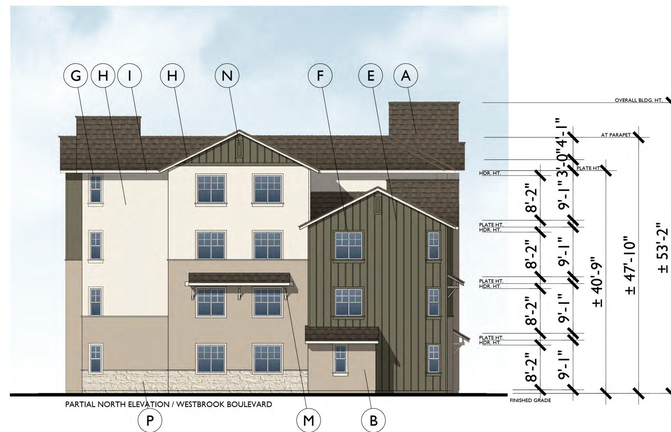
PARTIAL NORTH ELEVATION / WESTBROOK BOULEVARD
